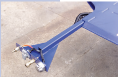
Simplified Hitching Swing-away connection module with air and electrical connections.
